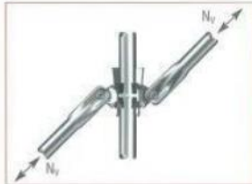
Axial force, diagonal brace
