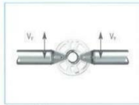
Horizontal shear force
